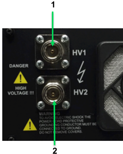
Fig. 3.3.2 HV connector , N-50/2-0/G1.07 type
